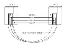
**NOTE**: Please do not use a "Swapped", "Flipped" or "Crossover" cable as it will not work with the ESCORT4580. To verify whether you have the correct type of cable, plug in the PSC04 (PL513). The red LED should turn ON. Connect the telephone cable to both the PSC04 (PL513) and the ESCORT4580 If the LED on the PSC04 (PL513) turns OFF and remains unlit, you are using the wrong type of cable.
